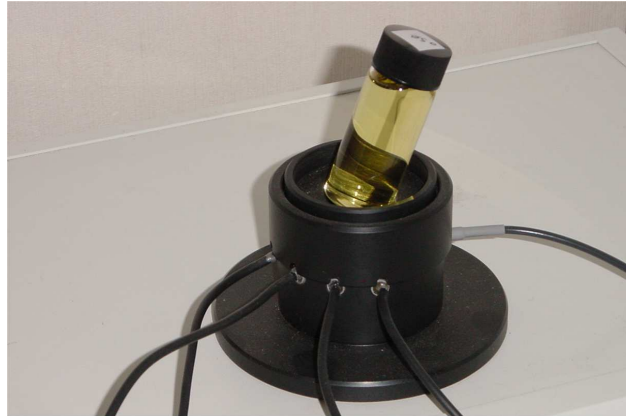
Fig. 4 - Optical probe for spectral nephelometry
